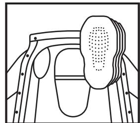
Make sure the back protector is oriented with its widest sheet of foam placed closest to the wearer's body.
