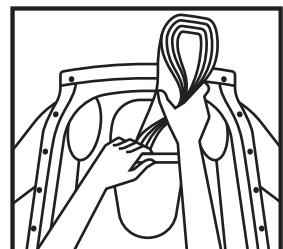
Insert the folded armor into the open velcro closure of the back armor pocket. The armor should fill out the entire pocket.
